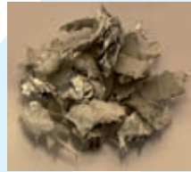
Granulated Floor heating pipe feed
