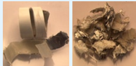
Floorheating pipes (pregrinding)
