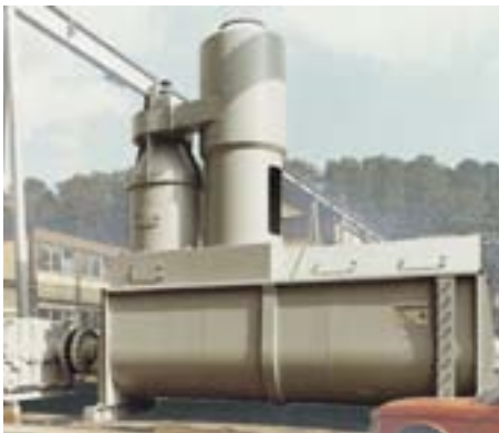
lime hydrator with wet scrubber
