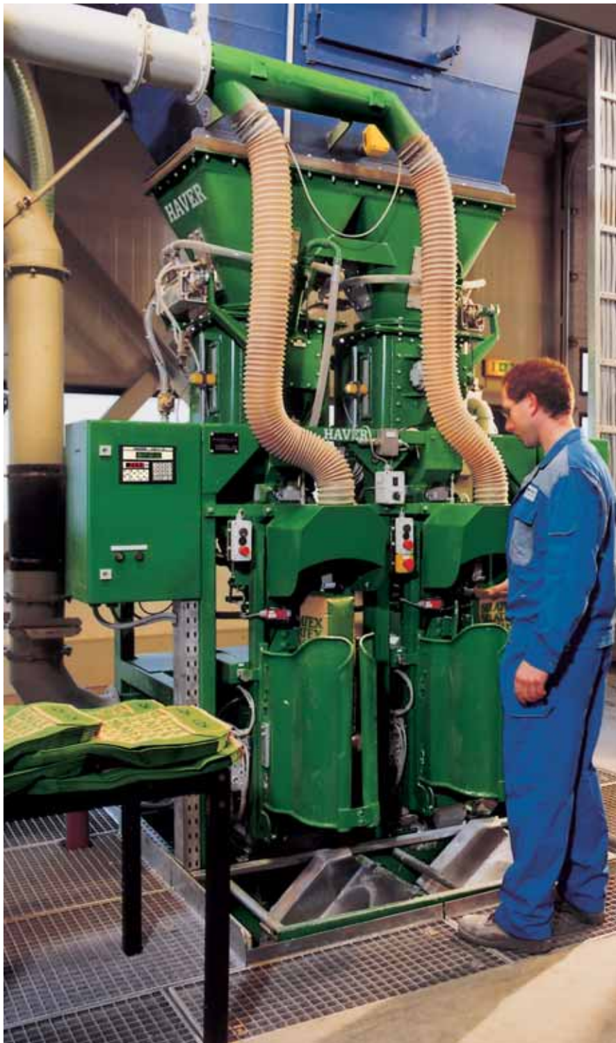
HAYER valve-bag filling machine using the air entrainment system outfitted with an automatic vertical bag discharger
