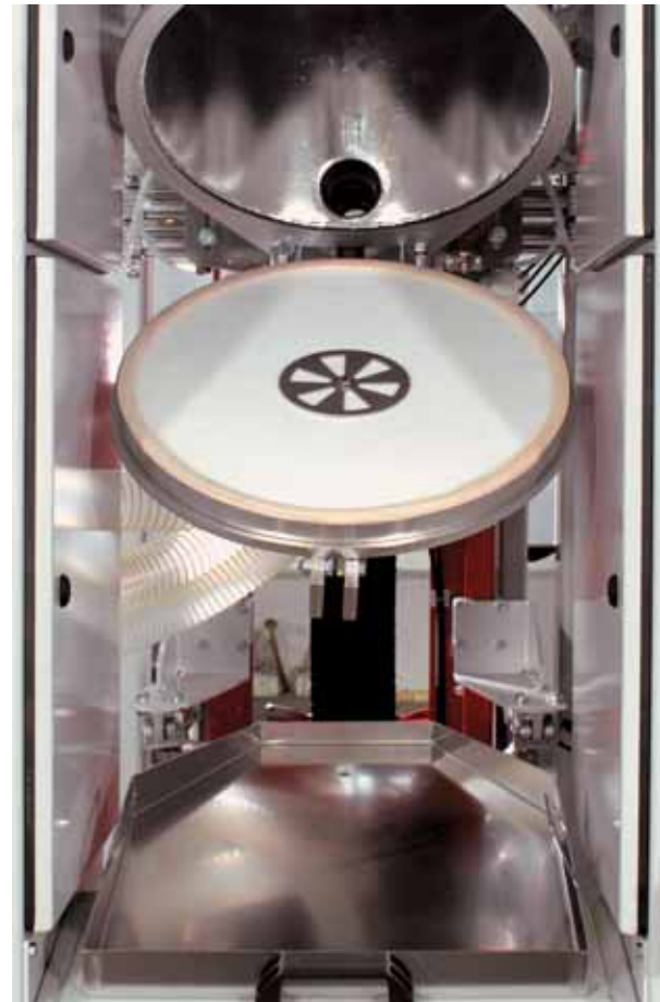
Opened pressure chamber allows easy and rapid cleaning
